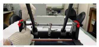
6.1.3 Pull up and turn over two handles to release two springs on the sides of the machine.
