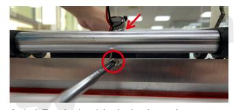
6.1.4 Push the blade lock and press the knife down. Remove the screw and spring on the back of the machine using a phillip screwdriver.
