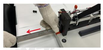
6.1.6 Pull out the old blade from the machine carefully and put it aside but with special attention. (1) Caution: Sharp blade!
